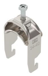
Clamp clip with U-foot, metal pressure trough with rounded edges to protect the cable. For vertical and horizontal mounting of 1 single cable on a C-profile rail. For slot width 18–22 mm. With 1-start screw thread on pressure trough, universal hexagonal screw head WAF10, with slot and cross recess. Suitable for mounting indoors and outdoors. We recommend the use of a counter-trough.
