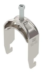
Clamp clip with U-foot, metal pressure trough with rounded edges to protect the cable. For vertical and horizontal mounting of 1 single cable on a C-profile rail. For slot width 18–22 mm. With 1-start screw thread on pressure trough, universal hexagonal screw head WAF10, with slot and cross recess. Suitable for mounting indoors and outdoors. We recommend the use of a counter-trough.
