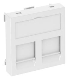
Data technology support with straight outlet and locking slider to accept two data technology connection modules with RJ45 socket. The locking fastening is suitable for horizontal and vertical installation in the system environment. Type C has a mounting opening of  $19.30 \times 14.80$  mm and is designed for direct fastening of the data connection modules in the mounting opening.
