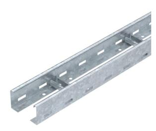
Cable ladder with a 60 mm side height with welded C30 profile rungs which are open in an upwards direction. Rolled side rail for reinforcement and as edge protection. Fastening to the bracket takes place using hold-down clamps, type LKS 40. The slot dimension of the rung is 16.5 mm and the appropriate clamp clip is type 2056.
