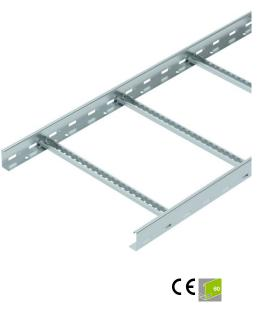
Cable ladder with a 60 mm side height with welded C30 profile rungs which are open in an upwards direction. Rolled side rail for reinforcement and as edge protection. Fastening to the bracket takes place using hold-down clamps, type LKS 40. The slot dimension of the rung is 16.5 mm and the appropriate clamp clip is type 2056.
