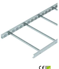
Cable ladder with a 60 mm side height with welded C30 profile rungs which are open in an upwards direction. Rolled side rail for reinforcement and as edge protection. Fastening to the bracket takes place using hold-down clamps, type LKS 40. The slot dimension of the rung is 16.5 mm and the appropriate clamp clip is type 2056.
