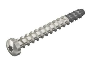
Stainless steel screw-in anchor for direct mounting without additional anchors in cracked and uncracked concrete and masonry. With round head for universal fastenings in wet rooms and outdoor areas. Torx drive T30.
