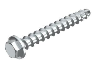
Bolt tie for direct mounting without additional anchors in cracked and uncracked concrete and masonry. With hex head drive and pressed washer to accept large loads. Suitable for fastening suspended loads from suspended supports and wall brackets.
