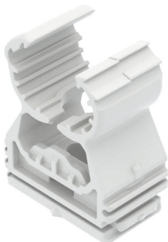
Highly stressable clip for accepting plastic or metal electrical and sanitary pipes as well as the electrical installation pipe Quick pipe. Universal fastening options on walls, ceilings and steel constructions, both indoors and outdoors. Flexible clamping range of several millimetres. Toolless pipe mounting. Connectable to each other to  $\varnothing$  32 mm, also with the OBO Quick or Multi Quick clip. For variable distances and clip quantity mountable on a profile rail.
