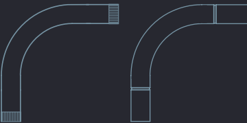
90° pipe bend with and without thread
