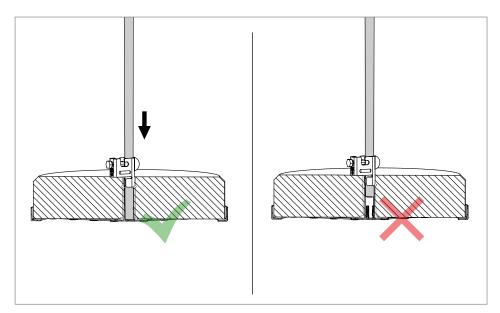
Fig. 5: Mounting the air-termination rod
