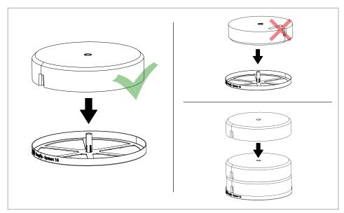
Fig. 3: Placing the FangFix concrete block on the base
