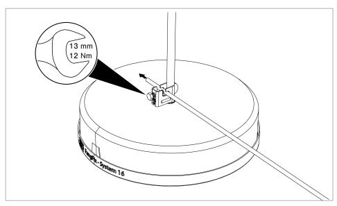
Fig. 6: Connecting the round conductor
