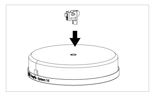
Fig. 4: Mounting the FangFix clamp
