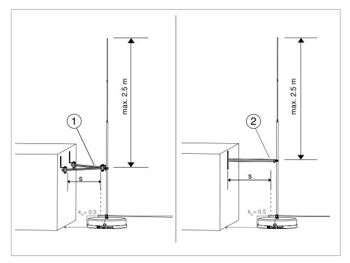
Fig. 2: Mechanical fastening of the air-termination rod
