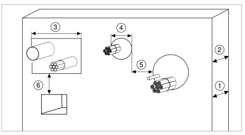
Fig. 2: Insulation distances to other components or component openings
