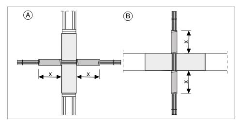
Fig. 4: Measure: FSB-WB 1.5 fire protection coil in wall A and ceiling B
