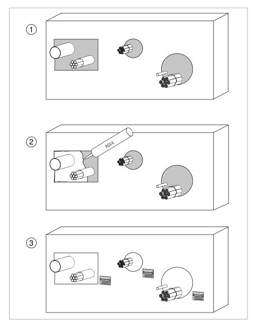
Fig. 10: Mounting small insulation
