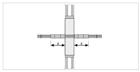
Fig. 7: Measure: Path insulation in wall
