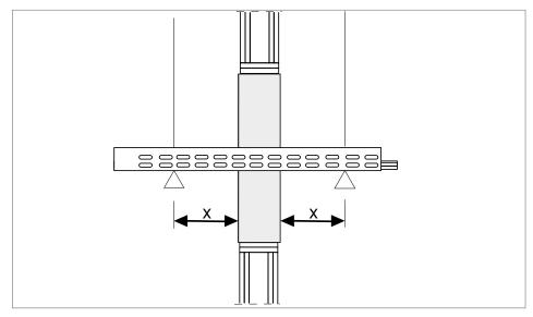
Fig. 3: Maximum distance for supports
